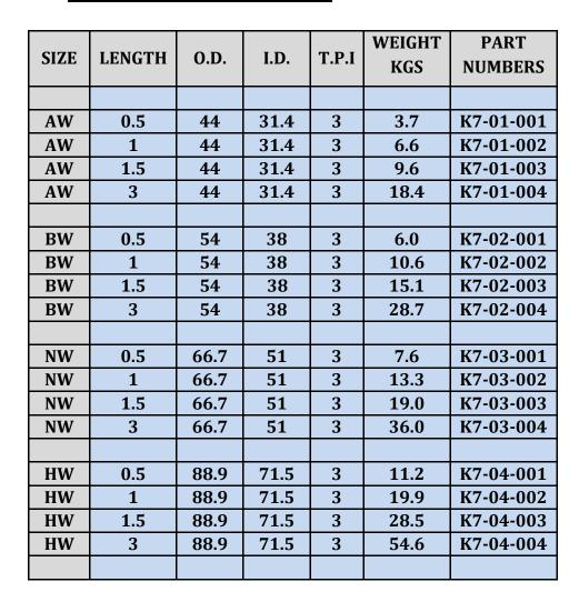
ALL AMKO DRILL RODS ARE MANUFACTURED FROM THE HIGHEST QUALITY RAW MATERIALS i.e. COLD DRAWN SEAMLESS TUBES OF GRADE SAE 1541 THAT ARE IMPORTED . THESE HAVE **EXTREMELY HIGH MECHANICAL PROPERTIES AND STRAIGHTNESS BETTER THAN 1: 2000. ALL DRILL RODS ARE PARALLEL WALL.**
